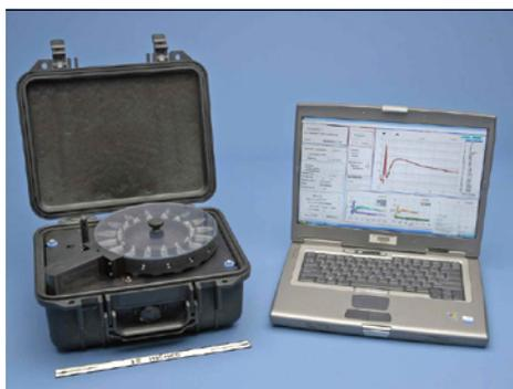
For liquid samples, the Laboratory developed a 16-channel sensor that processes ~100 samples in an hour. This unit has higher throughput than that of any competing technology.
