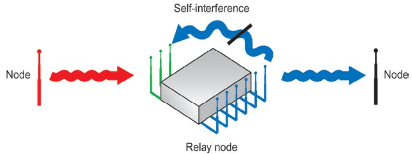
Figure 2. A full-duplex relay employing self-interference mitigation may provide the ability to build full-duplex nodes that simultaneously transmit and receive at the same frequency.
