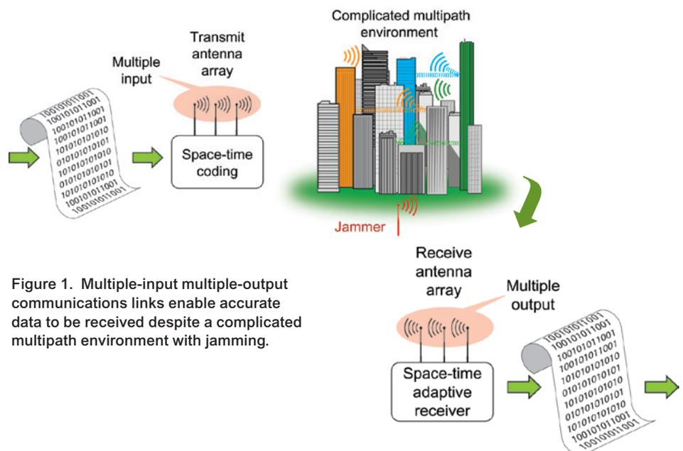
Figure 1. Multiple-input multiple-output communications links enable accurate data to be received despite a complicated multipath environment with jamming.
